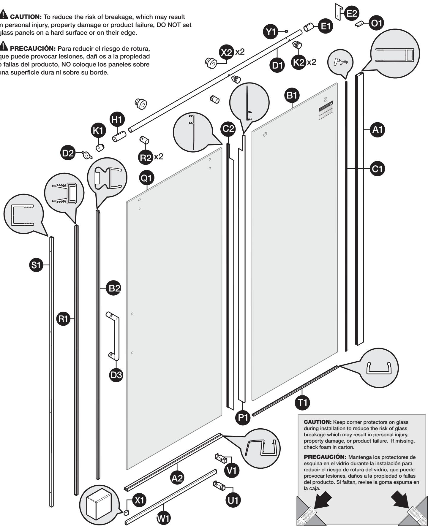
**CAUTION:** Keep corner protectors on glass during installation to reduce the risk of glass breakage which may result in personal injury, property damage, or product failure. If missing, check foam in carton.
