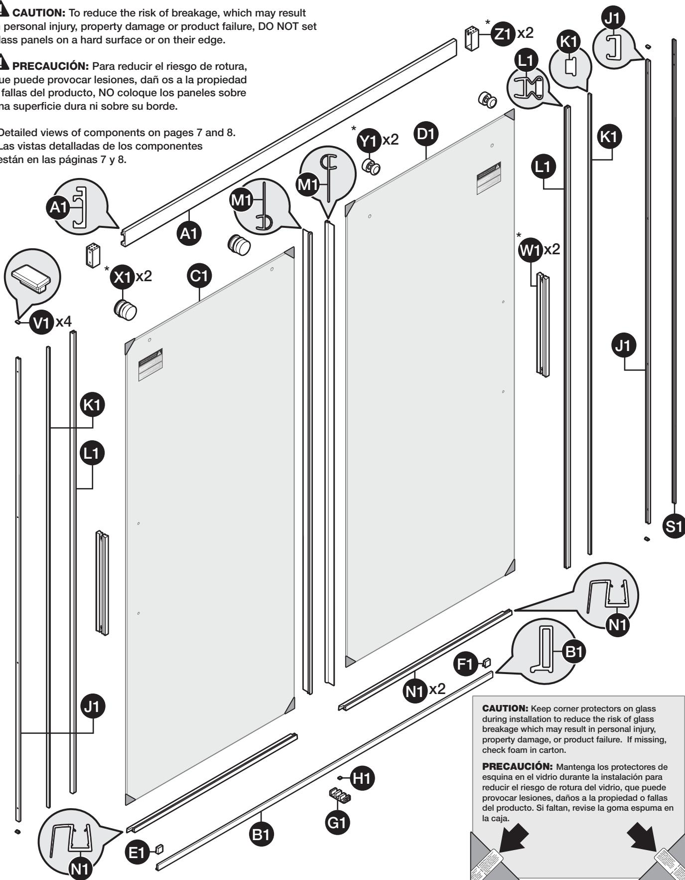
**CAUTION:** Keep corner protectors on glass during installation to reduce the risk of glass breakage which may result in personal injury, property damage, or product failure. If missing, check foam in carton.
